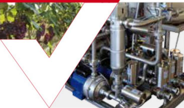
The crossflow filtering plant model CF is the result of the experience of Enoveneta in the membrane separation processes. The new crossflow filter is suitable for must, still wine, sparkling wine and wine with turbidity up to 1000 NTU (up to 2000 NTU with option prefilter) with a total maximum pressure of 8 bar (Isobaric line pressure + plant pumps pressure).
